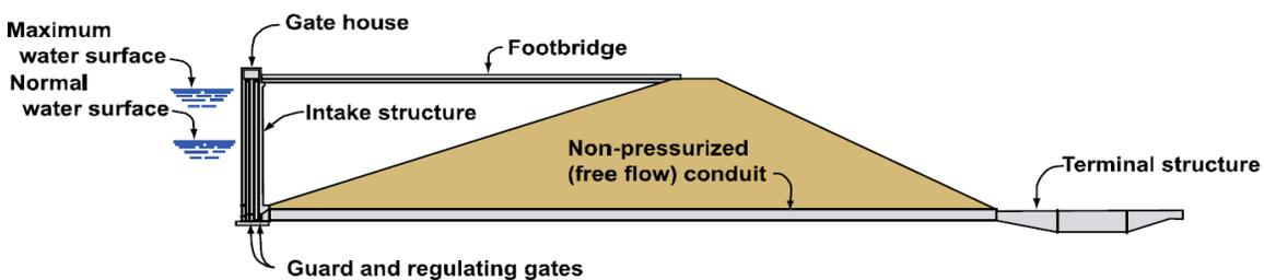
**Figure 1.** Upstream Control (Figure from FEMA 2005b).
