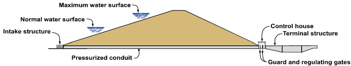
**Figure 2.** Downstream Control (Figure from FEMA 2005b).
