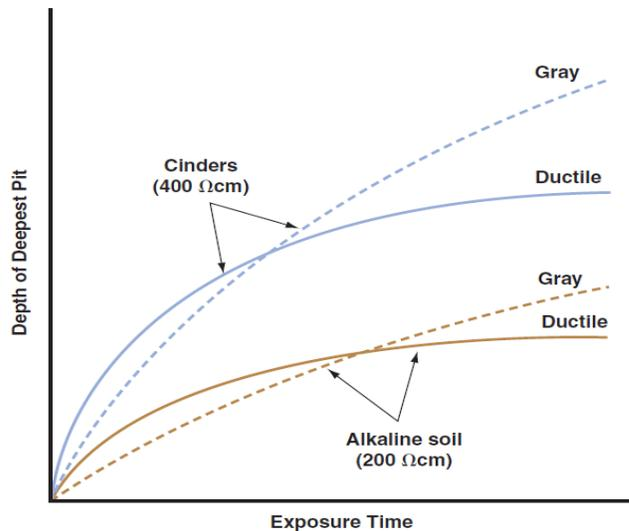
**Figure 4.** Increases of Maximum Pit Depth with Time for Ductile and Gray Pipes Buried in Two US Sites (Figure from Bonds et al. 2005).
