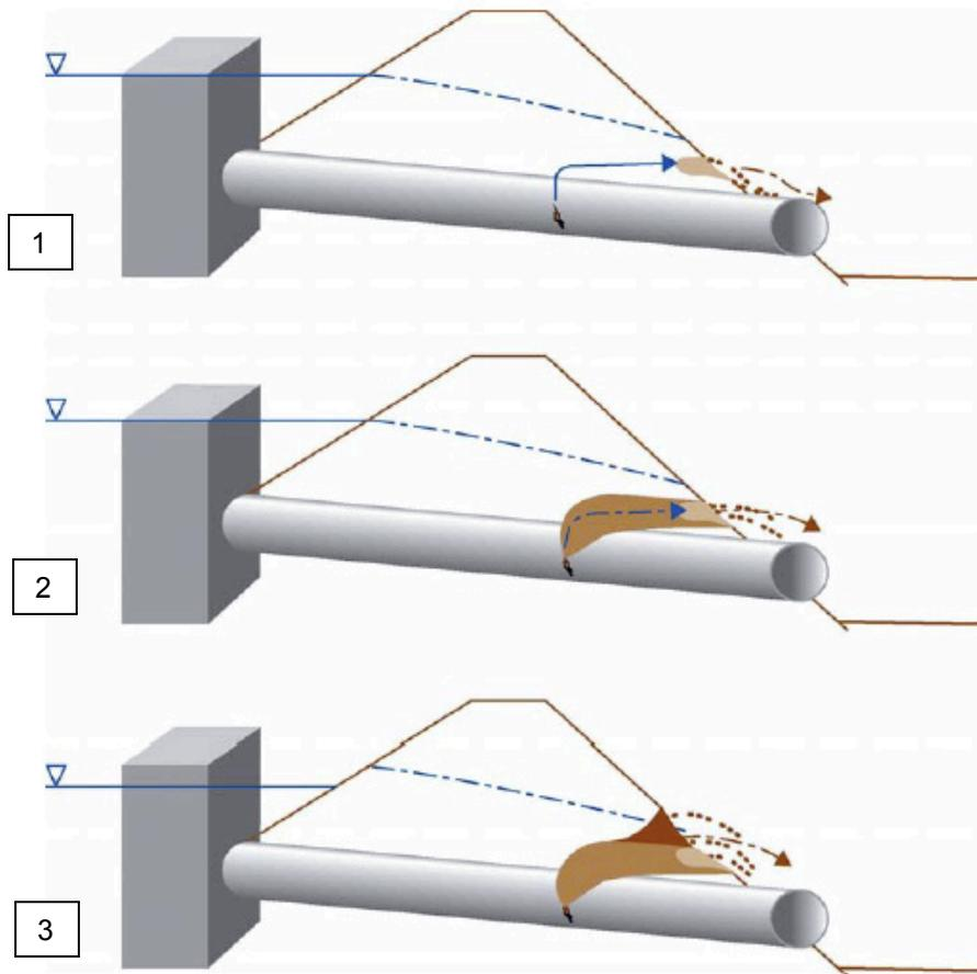
**Figure 3.** PFM 2 – Sequence of Backward Erosion Piping or Internal Erosion of Soils Surrounding a Pressurized Conduit with a Defect (Figure from FEMA 2005b).
