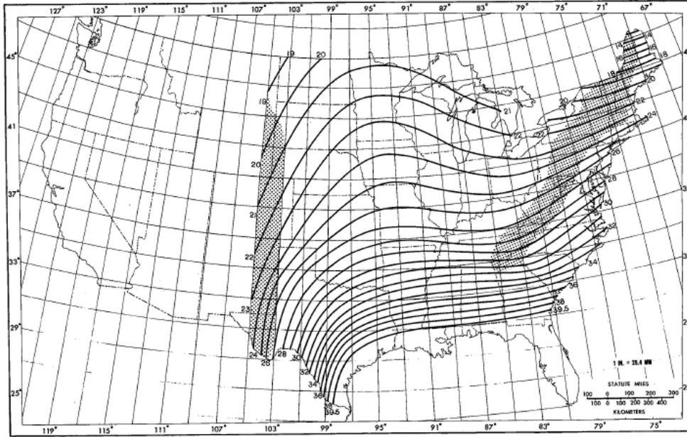
**Figure 3.** 24-Hour Duration, 200 square mile Drainage Basin All-Season Probable Maximum Precipitation Values (Obtained from HMR 51)
