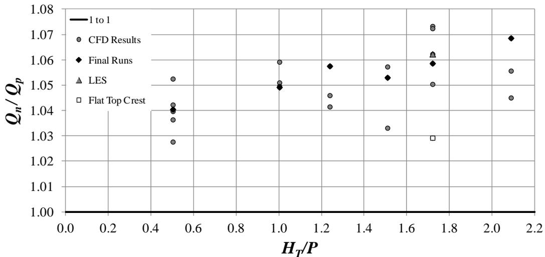
Fig. 4 – Agreement between  $Q_n$  and  $Q_p$  for  $15^\circ$  quarter-round trapezoidal labyrinth weir
