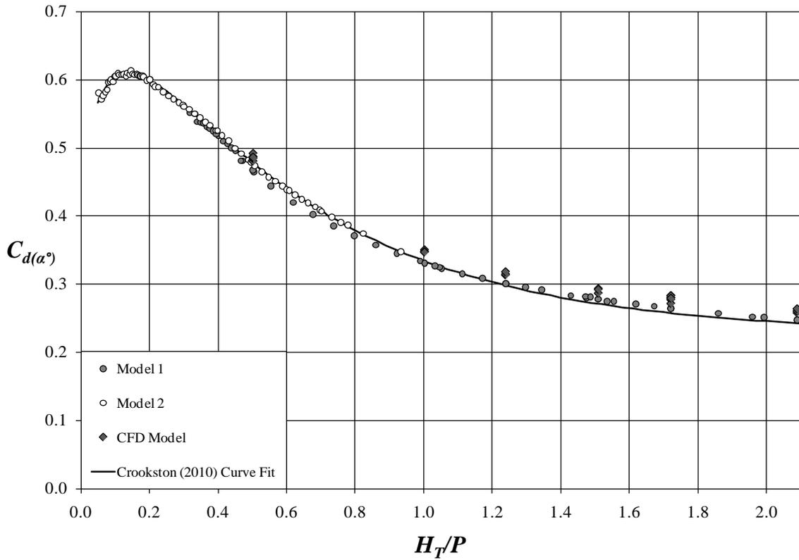
Fig. 3 -  $C_{d(\alpha^\circ)}$  vs.  $H_T/P$  for  $15^\circ$  quarter-round trapezoidal labyrinth weir, including preliminary numerical model results
