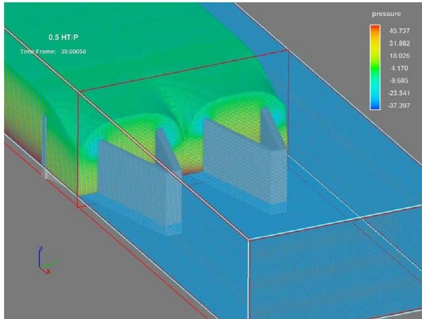
Fig. 2 – Numerical model, including computational mesh, boundary surfaces, and simulated fluid
