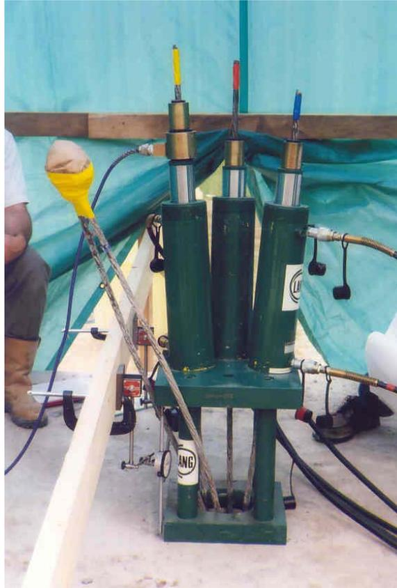
Figure 5. Sacrificial test anchor stressing jack.
